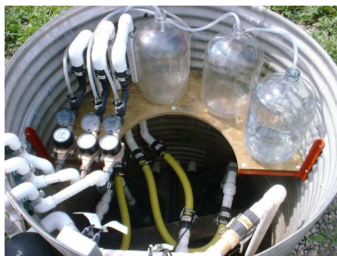
Figure 3. Drainage monitoring sump configuration
